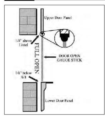
■ Locate the Door Panel Gauge Angle. Verify that the length of the Door Panel Gauge Stick equals the opening height of the door panels plus 1/4" (6mm)
