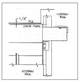
After installing the Lower Door Panel, install the Upper Door Panel following Steps 1 through 4 above. Hoist the Upper Door Panel into an Open position that is level from side-to-side and 1/8" (3mm) above the lintel. The Upper Door Panel should remain suspended from your hoist until door chain rods and chains are fully installed.
