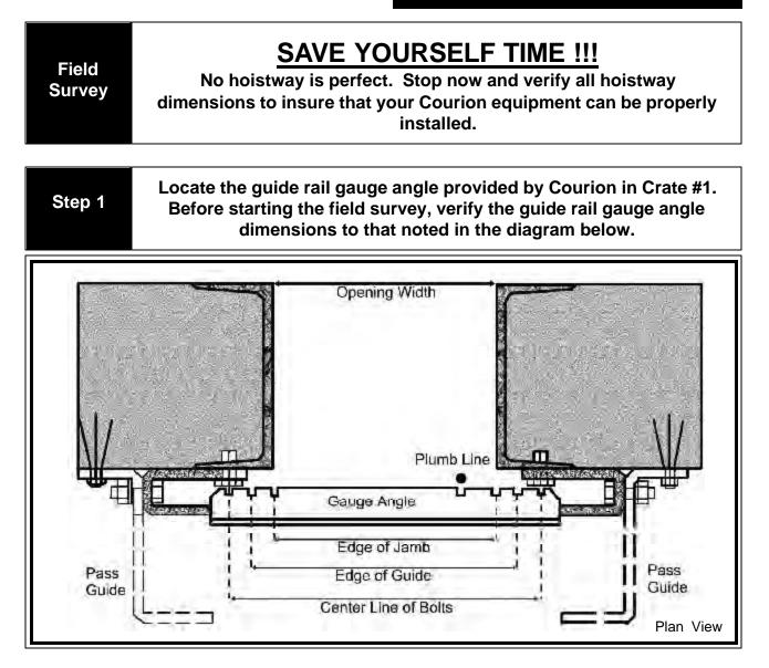
The guide rail gauge angle contains three (3) factory-made marks at each end:
