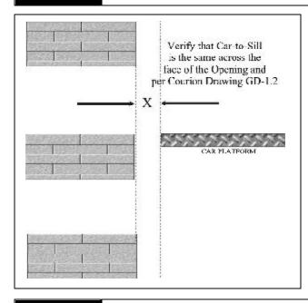
■ If the jambs are not plumb, use the shortest distance from the car platform to the entrance sill as the plane for guide rail installation.
