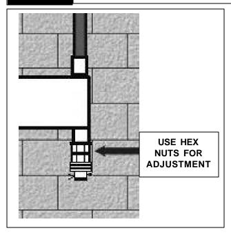
■ Apply weight to the LOWER DOOR PANEL to be sure that the door panels are in the FULL OPEN position and resting firmly on the guide or sill stops.
