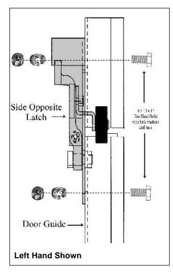
■ Using two (2) 1/2-13 x 1" Hex Head Bolts, lock washers and hex nuts found in Hardware Kit #135, attach the SIDE OPPOSITE LATCH to the Door Guide Rail on the side directly opposite the Interlock.
