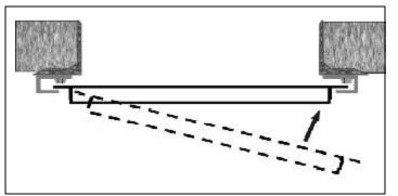
Step 3 Courion certifies the flatness of every door panel prior to shipment. However, shipping and job site handling may produce some twist or bow in the door panel. Check each Door Panel for flatness prior to proceeding with installation.
