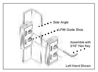
■ Using the 5/16-24 tapped holes provided in the Door Panel side angle, install four (4) **LF96 GUIDE SHOES**. The door shoe hardware is held captive in the Guide Shoe Assembly. Use a 3/16" allen (hex) wrench to loosely fasten the **LF96 GUIDE SHOES** to the Door Panel side angle.
