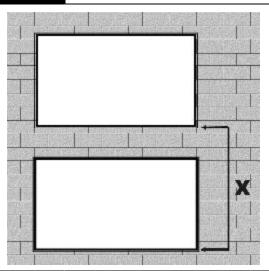
• Using a tape measure, verify that the actual floor to floor heights **(X)** are the same as that reflected on Courion Drawing GD-1.2.
