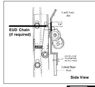
■ Drill a 5/8" (16mm) hole through the hoistway wall. This hole should be aligned as closely as possible to the hole in the top of the Interlock Roller Arm.
