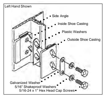
■ Using the 5/16-24 tapped holes provided in the Door Panel side angle, install four (4) **CAST GUIDE SHOES**. The INSIDE and OUTSIDE Shoe casting MUST be installed as shown or castings will move away from the Door.
