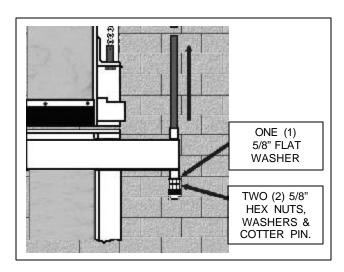
■ Thread two (2) 5/8" Hex Nuts onto the bottom of the CHAIN ROD. Locate the Hex Nuts slightly above the hole provided for the cotter pin. Be sure to install three (3) 5/8" Flat Washers between the cotter pin and Hex Nuts to keep the nuts from loosening.
