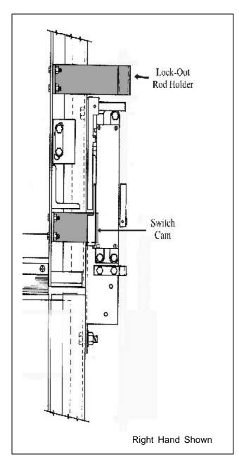
■ Using two (2) 5/16-18 x 1" hex head cap screws, flat washers, split lock washers, and hex nuts, attach the SWITCH CAM to the side angle of the Upper Door Panel using the pre-drilled holes provided by Courion.
