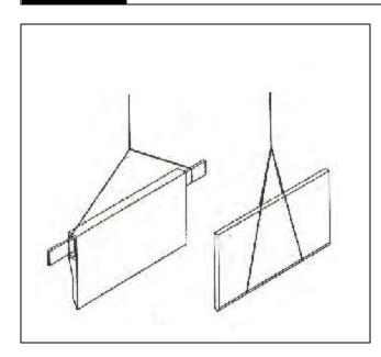
**IMPORTANT!** Be sure the hoist, hoist support, hoist chains, slings, straps, and any other accessories used to hoist the Door Panels into position are capable of safely supporting the Door Panels. Carefully inspect each component of the hoisting system for damage or wear before use.
