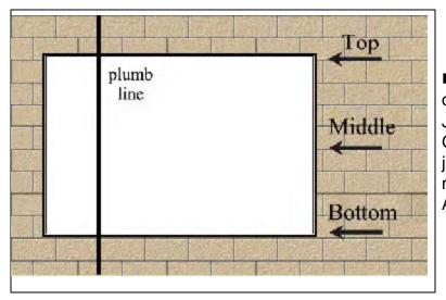
■ At the top, middle, and bottom of each opening, align the EDGE OF JAMB mark on the GUIDE RAIL GAUGE ANGLE with the edge of jamb and make a temporary chalk mark on the GUIDE RAIL GAUGE ANGLE at the plumb line.
