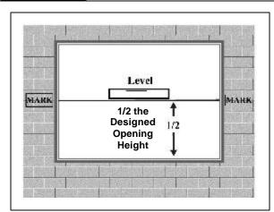
Using the GUIDE RAIL GAUGE ANGLE and level, make sure that the reference marks are level with each other.
