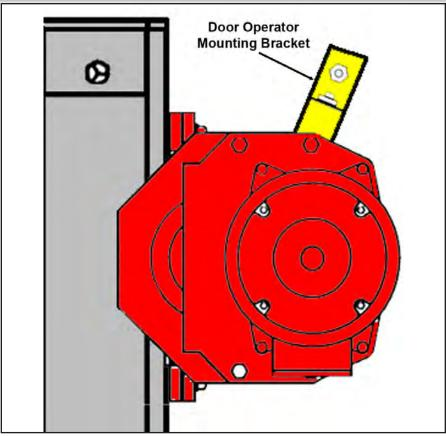
Attach the OPERATOR MOUNTING BRACKET found in Hardware Kit #30 to the outside corner of the Door Operator using one of the four bolts holding the operator casting together. Attach the other end of the Operator Mounting Bracket to the front hoistway wall using the sleeve anchor.
