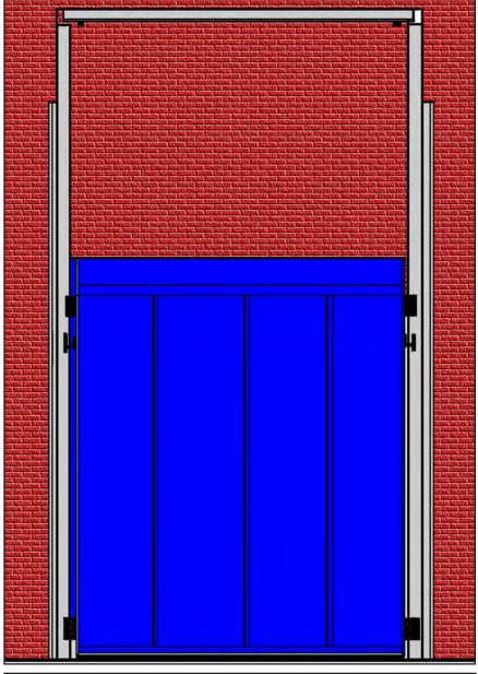
Courion checks each Door Panel for flatness prior to shipment. However, shipping and job site handling may produce some twist or bow in the Door Panel. Check each Door Panel for flatness by pushing the Door Panel against the guide bolts. If both shoe angles are flat against the guide bolts, twist is not present. If one side is not flat against the guide bolts, the Door Panel has some twist in it that must be removed before continuing with the installation.
