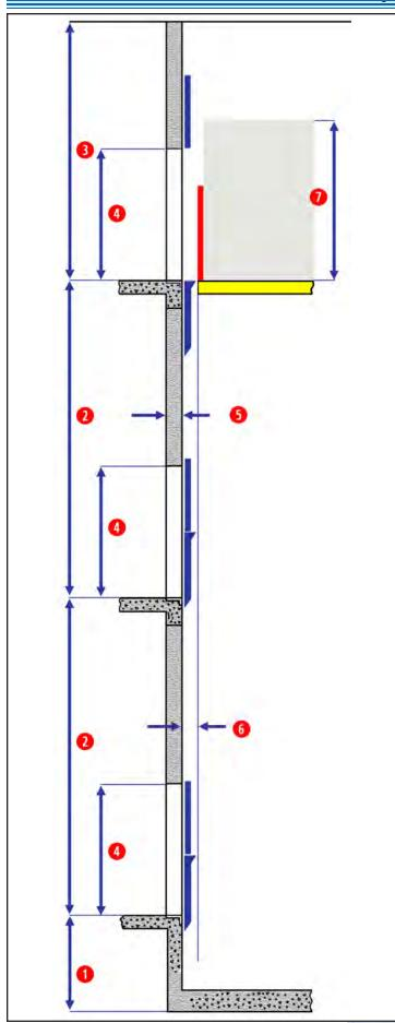
1 Pit Depth 2 Floor-to-Floor 3 Clear Overhead 4 Opening Height 5 Wall Thickness 6 Car-to-Sill Inside Cab
